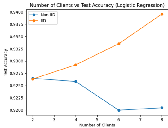
Figure 1: The influence of Number of Clients in Test Accuracy based on Logistic Regression model (Photo/Picture credit: Original).
