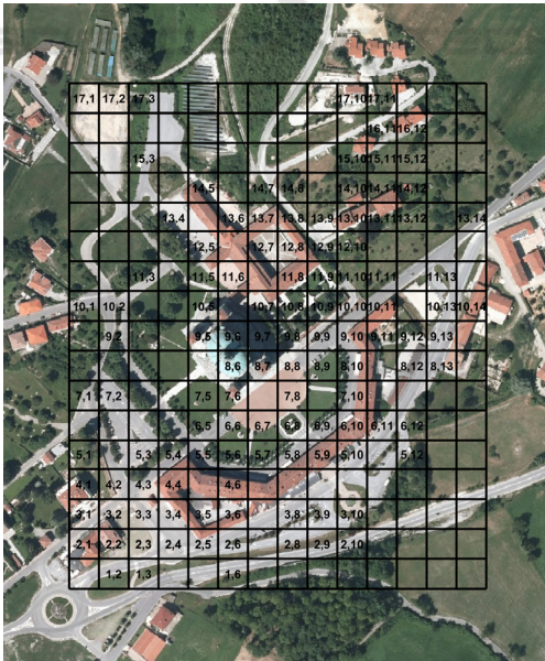
Figure 8: The grid created for the ROI has a cell size of 25 m. Each cell containing the PSs reports its index, represented by the number of rows and columns.
