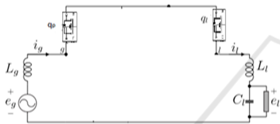
Figure 2(c): Mode 3 circuit of 5-level T-type inverter.
