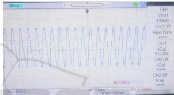
Fig 21: Input voltage for the proposed converter.
