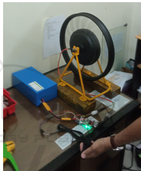
Figure 7: Motor Control Test with Thumb Throttle.
