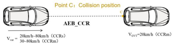
Figure 2. The test scene schematic of AEB CCR in C-NCAP.
