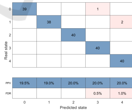
Figure 6. The classification effect on the gearbox fault dataset of Southeast University.
