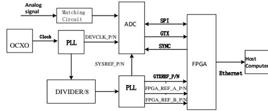
Figure 3. Hardware architecture.
