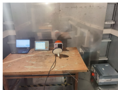
Figure 2: Beidou shipborne terminal system conducted disturbance test layout diagram.
