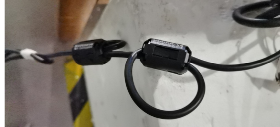
Figure 5: Electromagnetic compatibility rectification method—adding magnetic ring.
