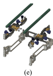
Figure 5: Robot structure design. (a) Ankle rehabilitation robot (b) Linear actuator (c-e) The moving platform of the rehabilitation robot.
