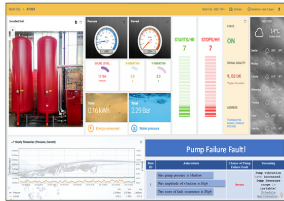
Figure 8: Individual telemetry unit's data with fault's explanation (Upasane et al., 2023).
