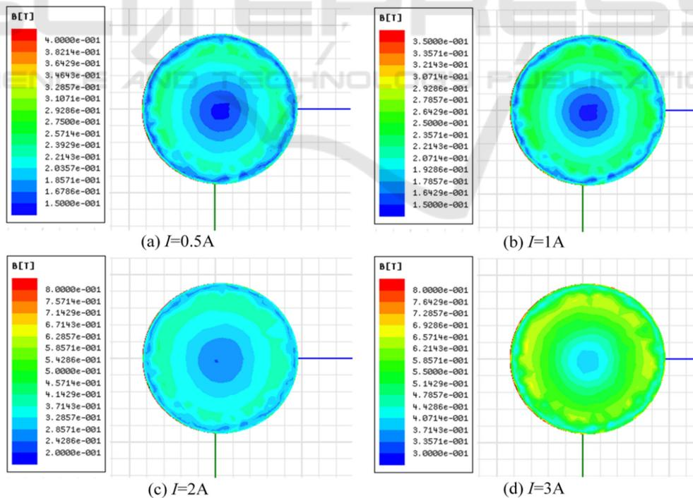
Figure 3: Distribution of magnetic flux density under different current.
