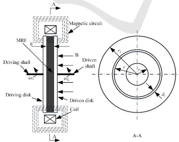
Figure 1: Working principle diagram of MRTD.
