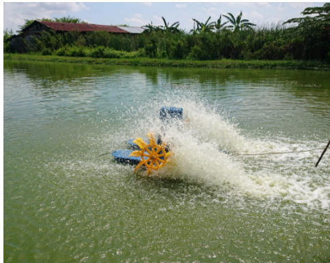
Figure 2. Pushing and splashing of water particles by paddlewheel operating in the pond.
