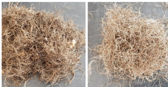
Figure 3: Steel wires extracted from used tyres.
