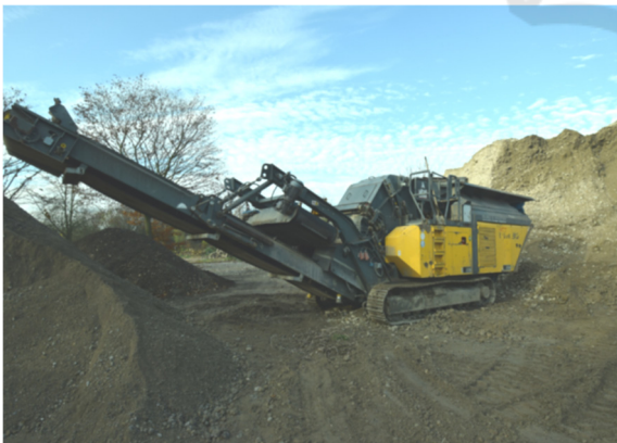
Figure 2: Processing and landfilling of the concrete rubble of the Pécs High-rise building.
