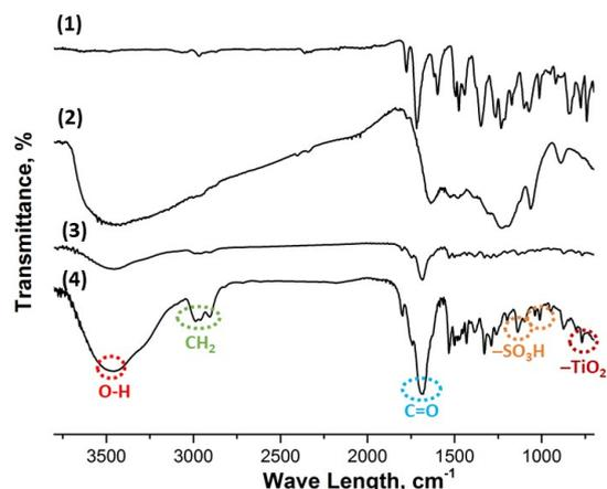
Figure 2: FT-IR spectra of (1) PEEK, (2) PES, (3) SPEEK and (4) PES/ SPEEK-TiO<sub>2</sub> membranes.
