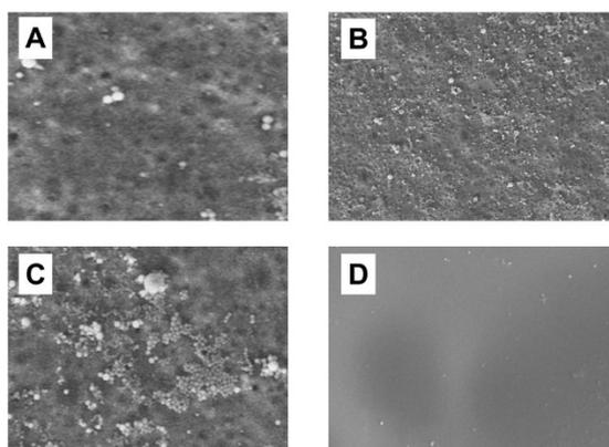
Figure 4: SEM image of (A) 20% SPEEK– 3% TiO<sub>2</sub>, (B) 20% SPEEK – 5% TiO<sub>2</sub>, (C) 20% SPEEK – 7% TiO<sub>2</sub>, (D) 20% SPEEK/3% PES – 5% TiO<sub>2</sub>
