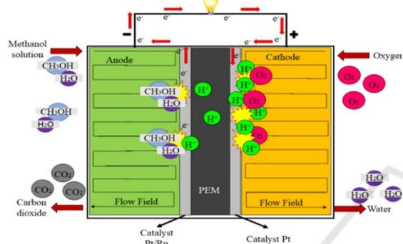
Figure 1: The fundamental composition of DMFC (Junoh, 2020).
