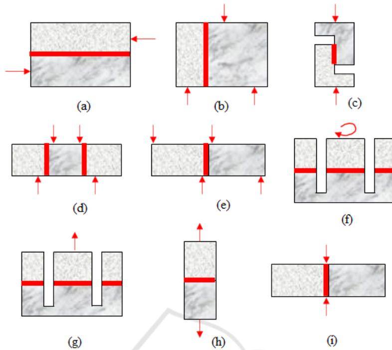
Figure 4: Shear test (a) – (f) and tensile test (g) – (i); (a) Mono surface shear, (b) Bi – surface shear, (c) push off (double L-shaped), (d) Direct double shear under JSCE, (e) FIP standard shear, (f) Twist - off.
