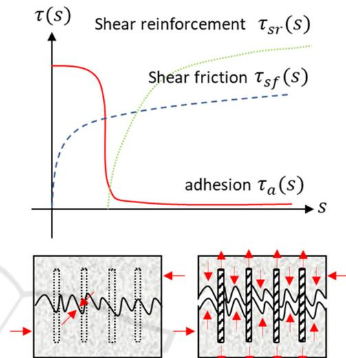
Figure 3: Load transfer mechanism of concrete to concrete – contribution of adhesion vs. shear friction vs. shear reinforcement (Lin & Erkut, 2013).
