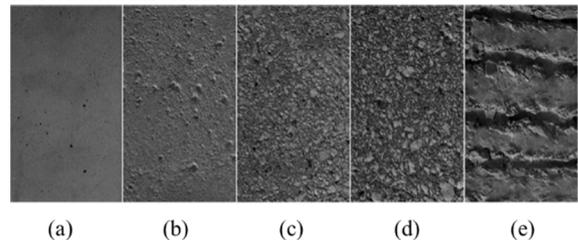
Figure 6: Surface preparation consists of the following steps: (a) casting; (b) wire brushing; (c) sand blasting; (d) shot blasting; and (e) hand scrubbing.
