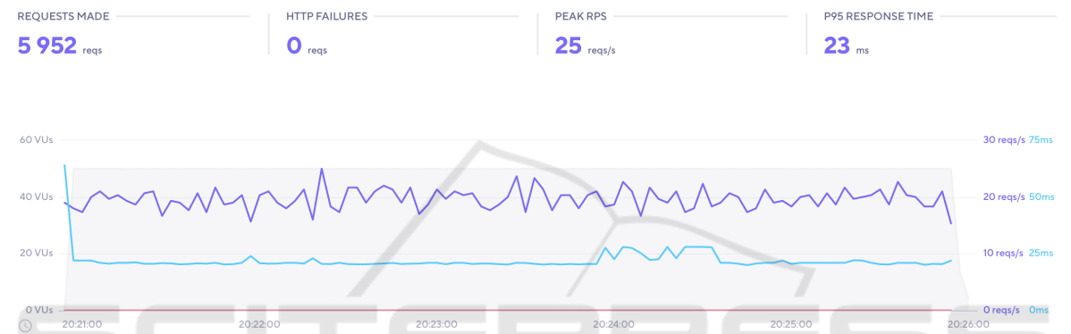
Figure 8: The response time when using TERA-Scaler.
