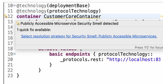
Figure 5: LEMMA Eclipse editor presenting the Customer Core operation model with security smell publicly accessible microservices.
