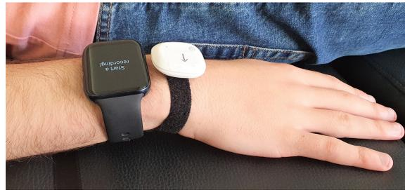
Figure 3: Setup used for the wearable devices attached to the wrist.
