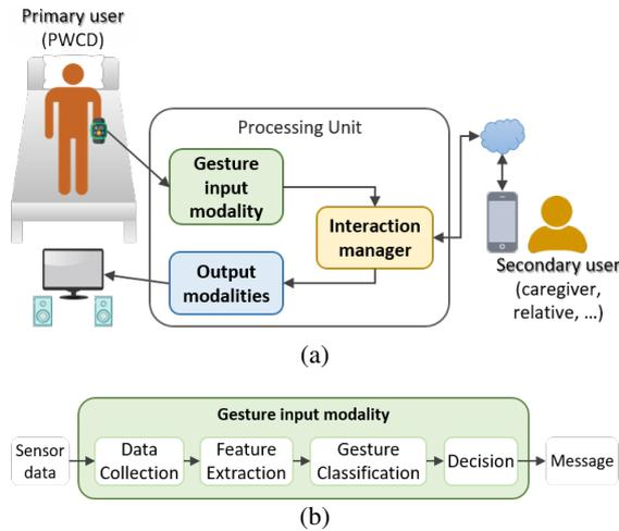
Figure 1: Overview of the proposed solution for communication support, including the users, sensors/devices, and interaction components (a), and main components of the gesture input modality (b).
