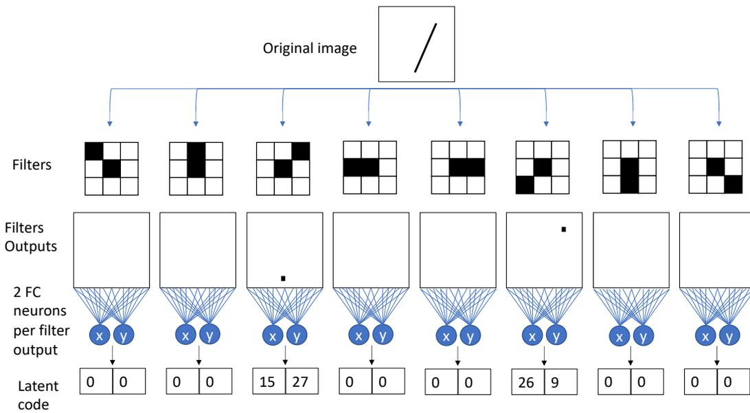
Figure 3: The encoder of AE2. It employs the 8 CNN filters to capture any line end configuration. See the explanation in the text.
