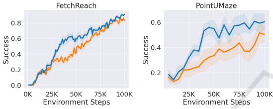
Figure 5: IMGEF agents with (blue) and without (orange) post-exploration. Left: Performance on FetchReach, with results averaging over 10 different random seeds. Right: Performance on PointUMaze, averaged over 10 different random seeds. Overall, agents with post-exploration outperform agents without post-exploration.
