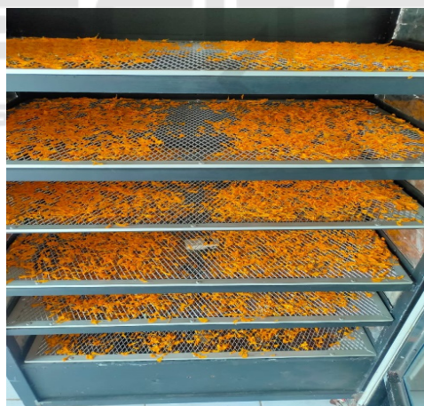
Figure 6: Gemitir flowers that have been dried for 24 hours in a dehumidification system dryer.
