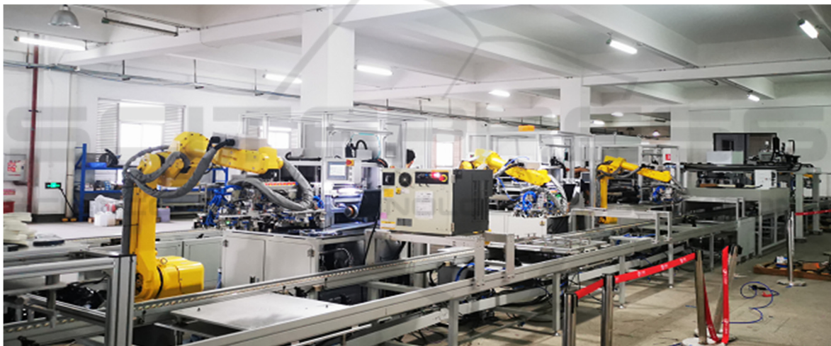
Figure 1: Application of an automatic processing method for shoe sole production and the adopted equipment
