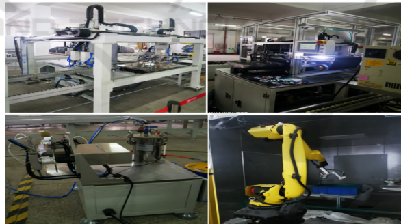
Figure 4: Automatic glue spraying, automatic hot printing, automatic film pressing, automatic sole cleaning and automatic wear-resistant spraying for the processing of shoe soles.
