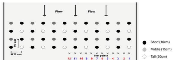
Figure 2: The layout of vegetation array and measurement locations in the downstream zone.
