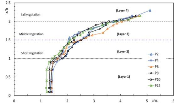
Figure 7: Velocity profiles behind the gap of vegetation for all positions.
