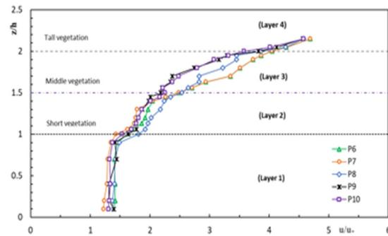
Figure 8: Comparison of velocity profiles at various positions behind the vegetation.
