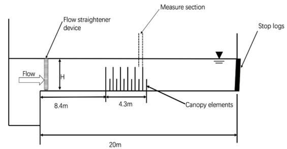
Figure 1: The sketch of the experimental flume.
