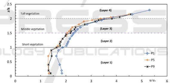
Figure 4: Velocity profiles directly behind the tall vegetation (Group B).
