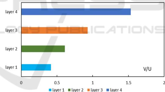
Figure 11: Averaged velocity ( $V$ ) of each layer for the half channel. Note:  $U$  is the cross-sectional mean velocity of the channel.
