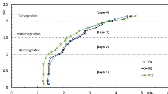
Figure 6: Velocity profiles behind the gap of vegetation (Group D).
