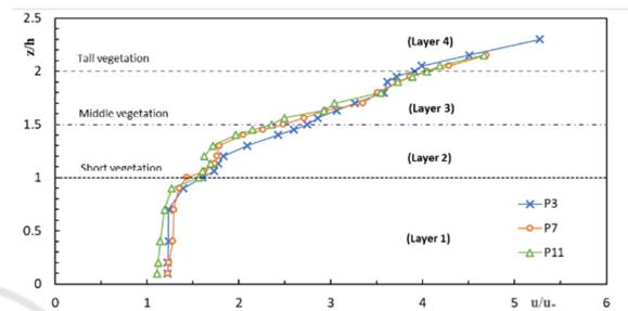
Figure 3: Velocity profiles directly behind the short vegetation (Group A).
