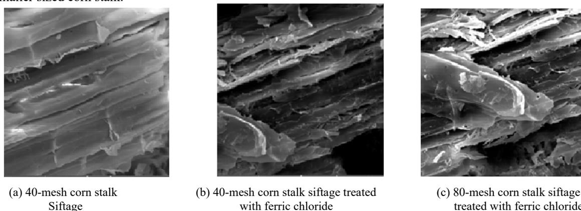
Figure 3: Electron scanning microscopy of the corn stalk raw material.
