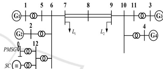
Figure 6: Four-machine two-area system structure diagram.
