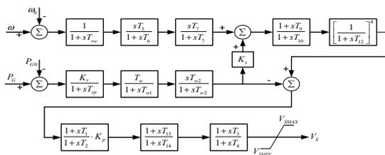
Figure 4: Model block diagram of SI PSS.
