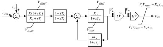
Figure 1: Model block diagram of FV excitation system
