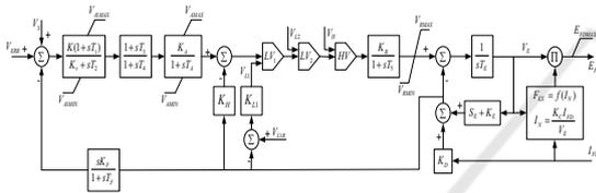
Figure 2: Model block diagram of FM excitation system.
