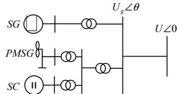
Figure 5: Single machine infinite bus system structure
