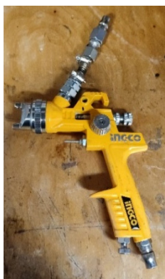
Figure 2: Spray gun for mixing oil and air.
