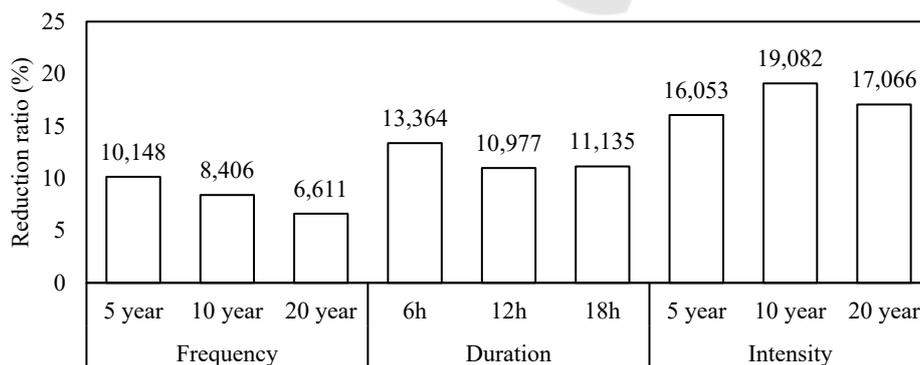
Figure 6: Reduction ratio of runoff coefficient under different rainfall characteristics.
