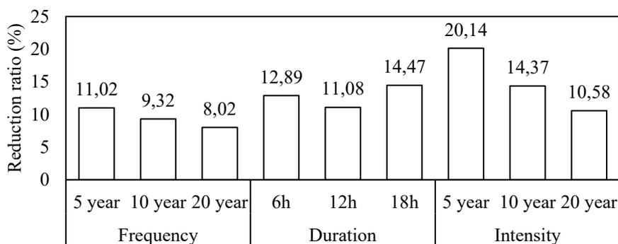
Figure 5: Reduction ratios of inundation areas under different rainfall characteristics.
