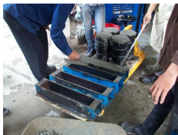
Figure 5: Concrete Casting Process.
