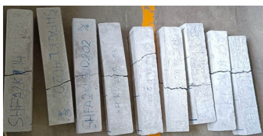
Figure 12: The Crack Pattern of Specimens After Flexural Testing.
