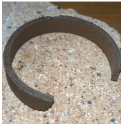
Figure 2: Finished product sealface ring formed by powder metallurgy technology (Fachrul Rozy, Kurniawan).
