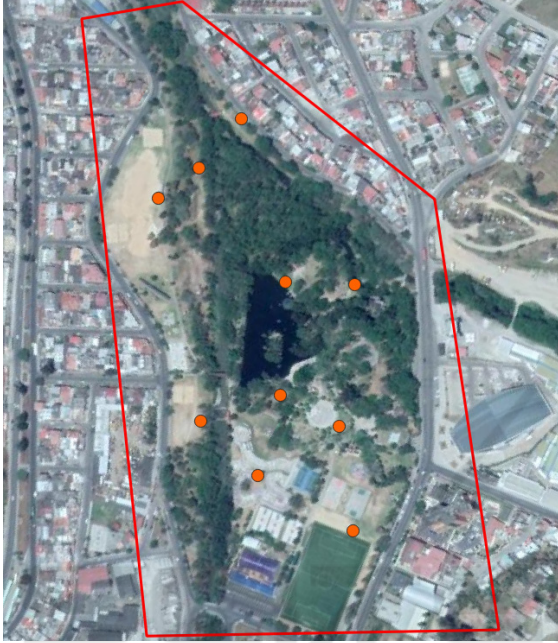
Figure 3: Delimitation of the zones in the urban area in the city of Loja and installation of the GCPs. This area corresponds to Jipiro.
