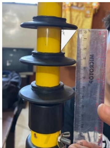
Figure 6: Rubber rings on 20kV shaft as safety.
