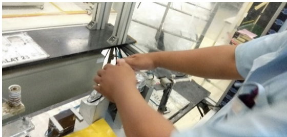
Figure 1: Manual Lens Pressing Process.
