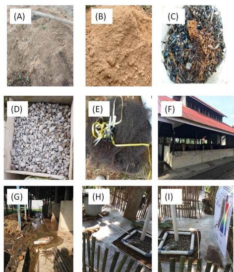
Figure 2: Materials for STBM system, Wastewater Source from Cattle Farm and brick type STBM system: (A) Local soil, (B) sawdust, (C) iron pellets, (D) split stone, (E) palm fiber, (F) Cattle farming (G) Wastewater from cattle farms, (H) STBM system brick arrangement (i) the STBM system is installed underground.
