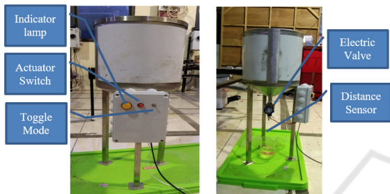
Figure 4: Automatic filling machine hardware.
