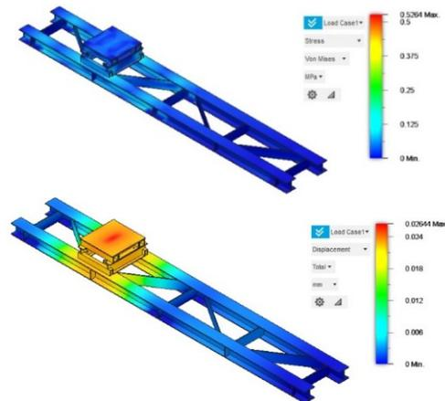
Figure 10: (a) Stress Result of Model 1; (b) Displacement Result of Model 1.
