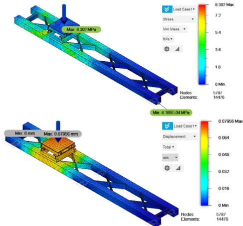
Figure 14: (a) Stress Result of Model 5; (b) Displacement Result of Model 5.
