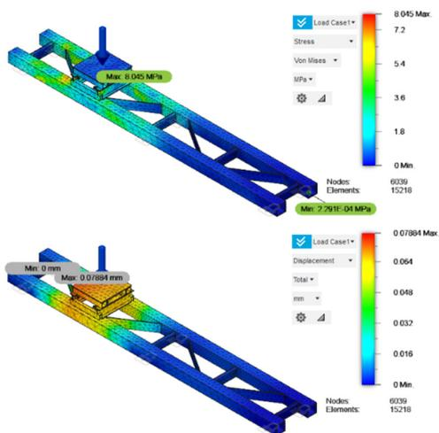
Figure 13: (a) Stress Result of Model 4; (b) Displacement Result of Model 4.
