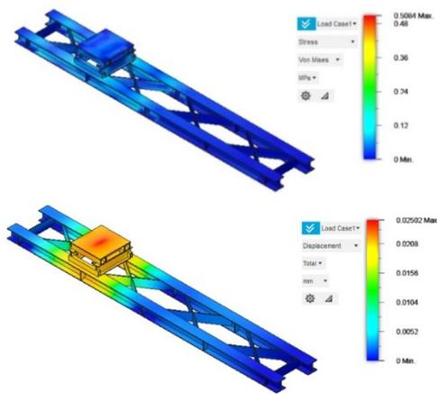
Figure 11: (a) Stress Result of Model 2; (b) Displacement Result of Model 2.
