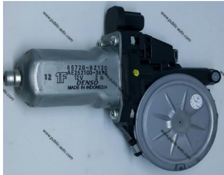
Figure 5: DC motor 48 watts.
