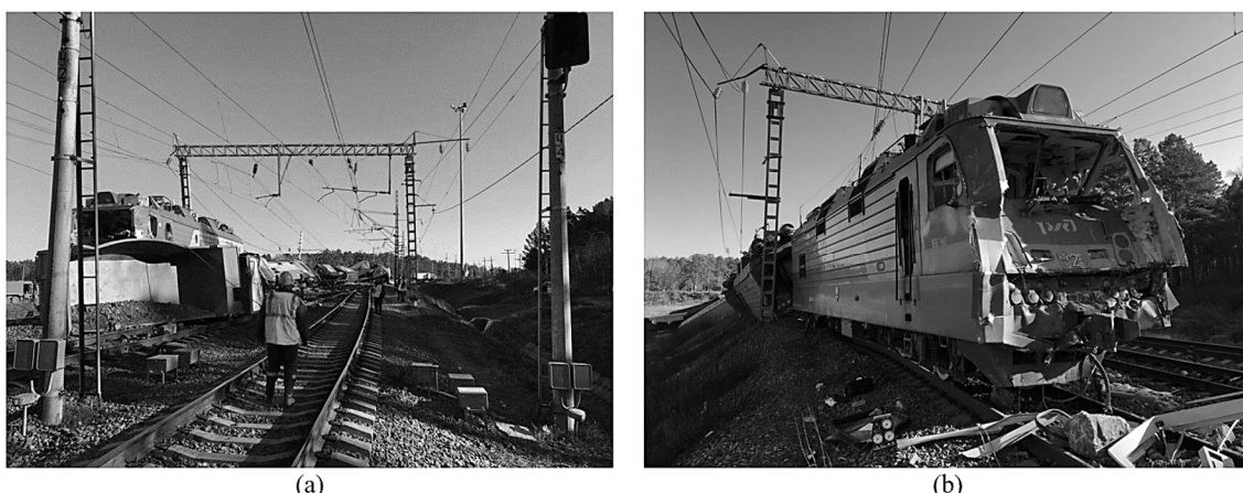
Figure 1: Consequences of the collision between 3ES5K (Ermak) electric locomotive and truck on October 23, 2021: (a) general view after the collision, (b) view of the cab of the electric locomotive after the collision.
