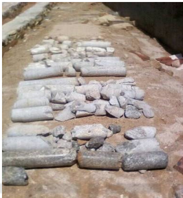
Figure 9. Drilling cores for 28m depth.
