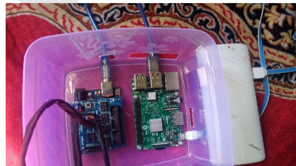
Figure 3: Heart rate and body temperature monitoring prototype (Inside Display).
