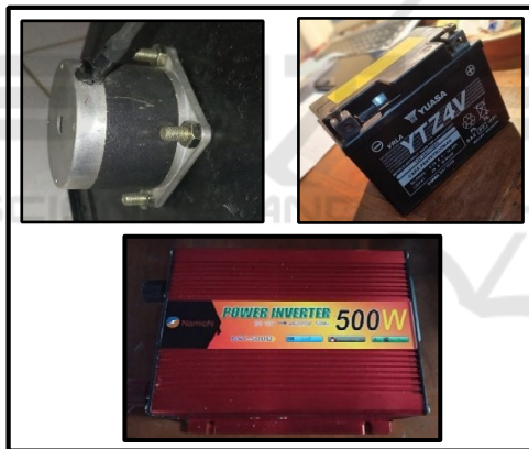
Figure 4: I Power generation components (generator, inverter, and battery).
