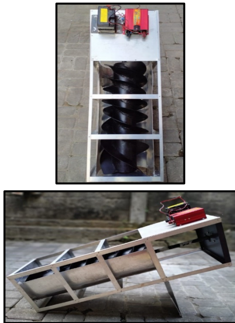
Figure 3: Prototype micro hydro screw Archimedes turbines portable.
