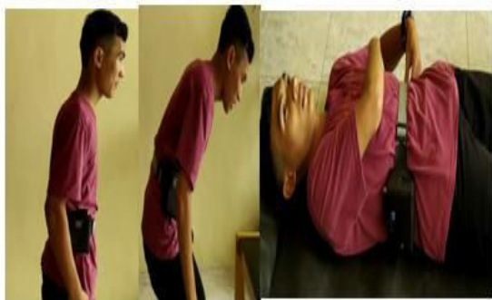
Figure 7: The implementation and testing of fall detection of vertigo and syncope patient.
