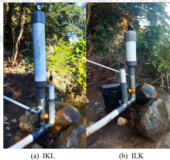
Figure 3: Schematic of the hydraulic ram pump test installation.
