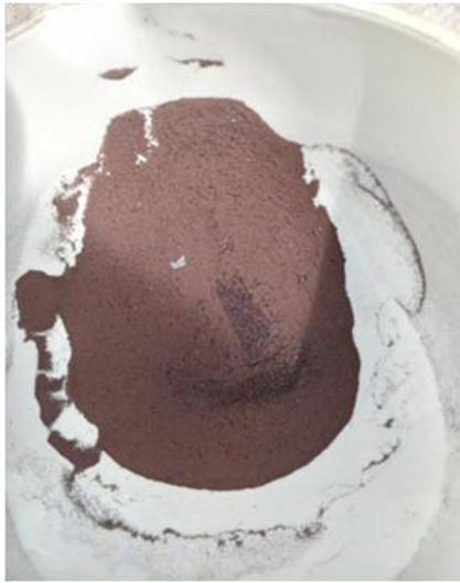
Figure 2: Copper Coated MWCNT's of a Brown Color.
