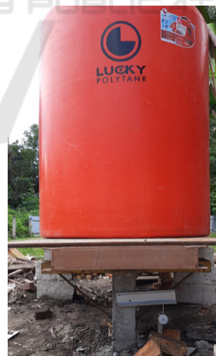
Figure 6: Static loading test of mini pile.
