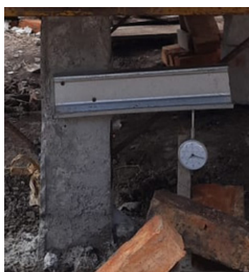
Figure 7: Recorder settlement using dial gauge.
