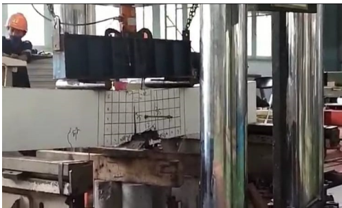
Figure 6: Specimen precast beam was under tested.
