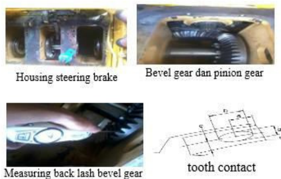
Figure 5: Install bever gear.
