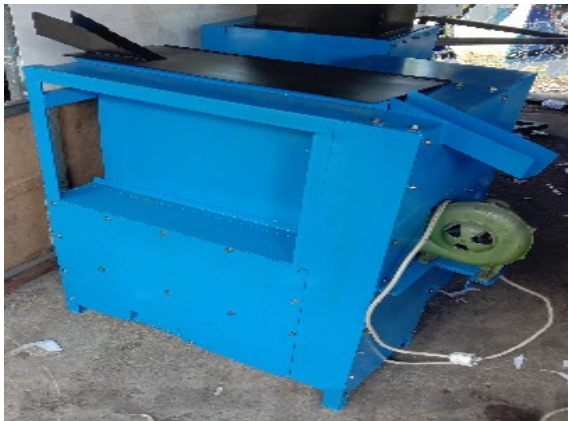
Figure 3: Corn Sheller Machine.
