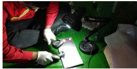
Figure 13: Test Specimen Defect Measurement.
