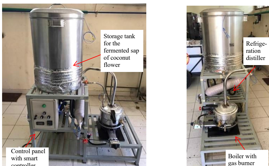
Figure 1: The established distillation machine completed with refrigeration distiller, smart controller and large storage tank for fermented sap of coconut flower.
